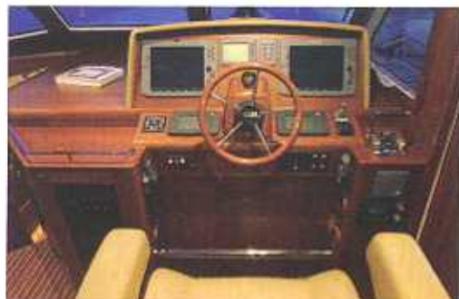
The redesigned helm, above, is new to Grand Banks owners, featuring a smaller wheel and a Stidd helm seat that slides back for standing operation. The amidships master, right, is perfect for long voyages with tons of storage and creature comforts.
