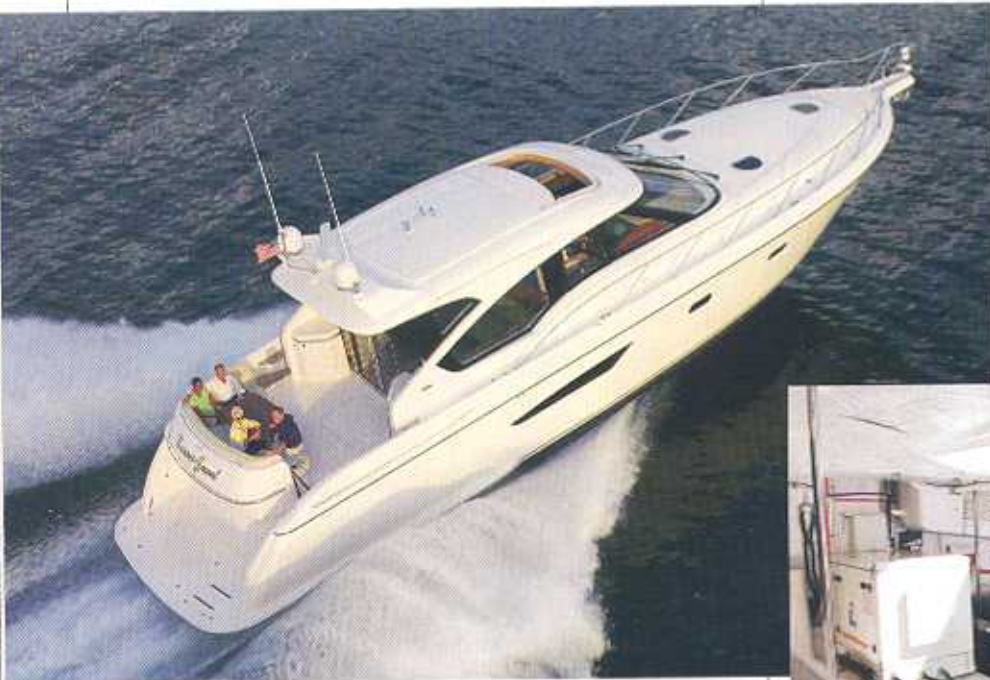
Tiara's new Sovran 5800 (above) is the first U.S.-built cruiser to be equipped with three IPS drives. The engine room (right) takes up little lineal space in the boat and provides plenty of access for maintenance of the Volvo diesels.
