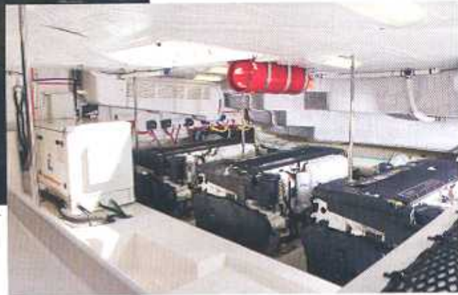
Tiara's new Sovran 5800 (above) is the first U.S.-built cruiser to be equipped with three IPS drives. The engine room (right) takes up little lineal space in the boat and provides plenty of access for maintenance of the Volvo diesels.
