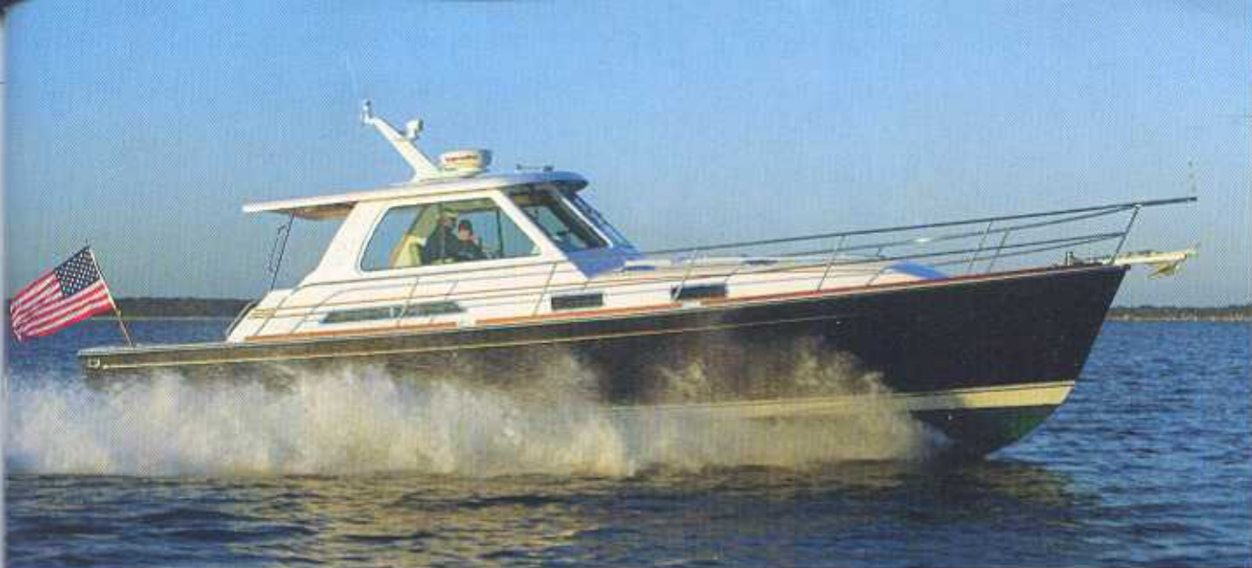
In 2008, Sabre's tried-and-true 42-foot express cruiser will be offered with twin Zeus drives, which — because they are mounted in the stern — will allow a bulkhead shift and permit enlargement of the living accommodations below.
